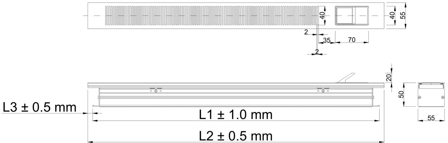
Figure 1: Ventiont SCW-SH dimensions
