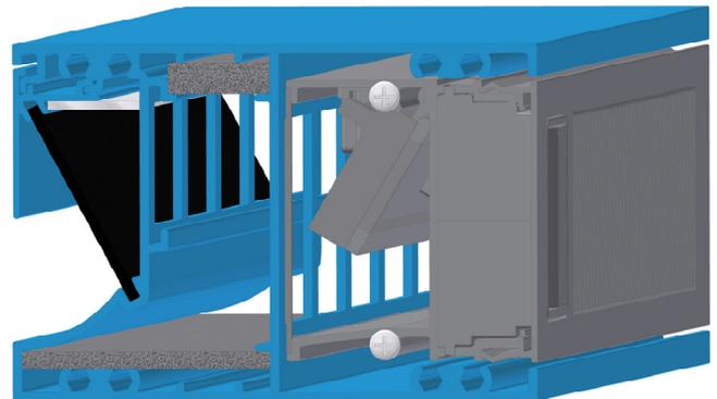
increased air-tightness of modern buildings requires consideration of sources of make-up air. Make-up air drawn through gaps and service penetrations does not meet the requirements of Clause 2.3 within the standard and can lead to the loss of amenity in the enclosure. Ventient SCW-SH could be an acceptable permanent natural ventilation opening as required in Clause 2.3.
